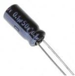
The capacitor has a short and a long leg, and a stripe on one side. Like LEDs, they must be connected with the short leg and stripe to negative (ground). We're using a 1 microfarad capacitor and you should too.
