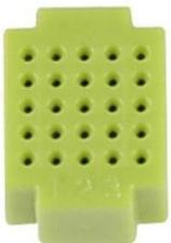
This micro breadboard has 25 connection points. The columns are numbered from 0 to 4 (some have the middle columns 1, 2 and 3 marked). All points on a column are connected together, but the different columns are not connected. You can use a larger breadboard if you wish.
